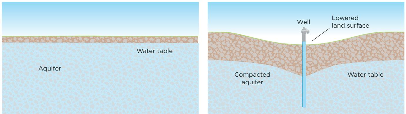
Chronic overdraft of an aquifer can lead to major problems by causing **land subsidence**, the settling or sinking of land. The rapid rate at which land is sinking in California puts infrastructure such as canals, pipelines, roads, and buildings at risk. This land loss is often irreversible. Recent US Geological Survey data show extraordinary land subsidence in the Central Valley, cracking a major water delivery canal and threatening to make it unusable (Sneed, Brandt, and Solt 2013).
