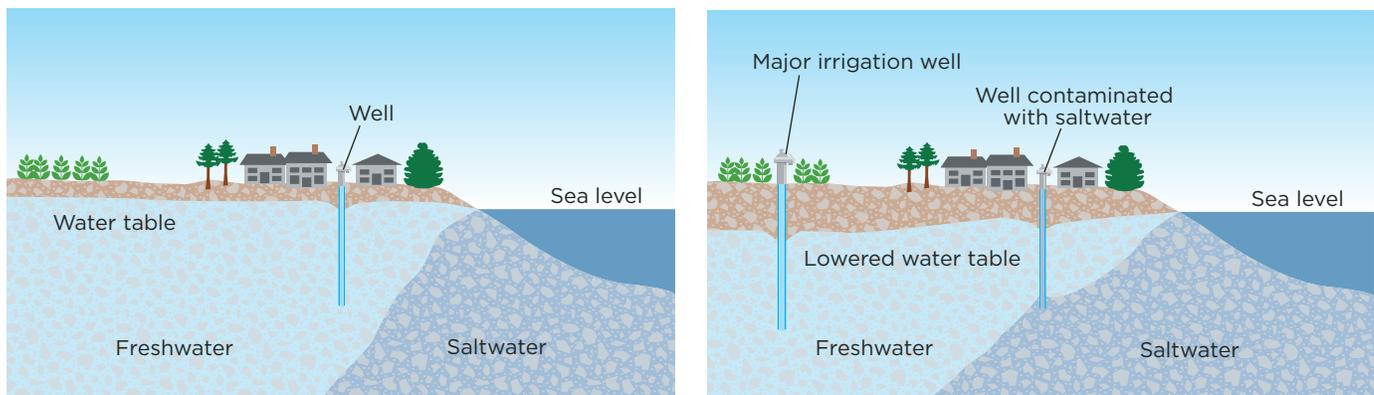
Freshwater is less dense than saltwater, and therefore floats on top of saltwater in an aquifer. When freshwater is pumped out of the aquifer, its weight on the saltwater is diminished, letting the saltwater rise and flow toward the source of the pumping. This can result in **saltwater intrusion** into drinking water and agricultural water supplies.
