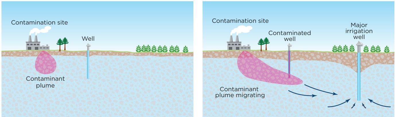
**Contaminant plumes** are a mixture of waste chemicals and groundwater that exist in the aquifer near the sites where they are produced. Groundwater pumping can pull a plume from its current location toward nearby wells, putting them at risk of contamination.
