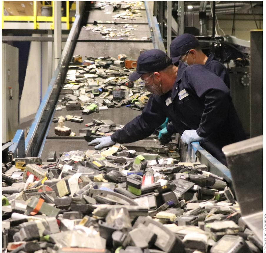
*Recycling the cobalt, lithium, and other critical materials in electric vehicle batteries will help meet increased demand for materials as vehicle sales grow in future years and reduce the need to mine new materials. Recycling facilities are currently few and far between—Li-Cycle (shown above) is one of just 10 or so in the world operating today—underscoring the need for policies to help promote increased recycling.*
