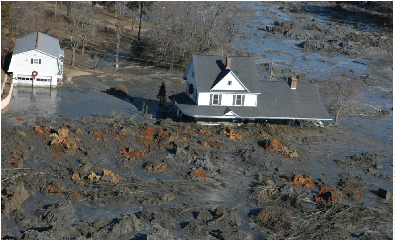
The largest industrial disaster in US history, the Kingston coal ash spill on December 22, 2008, destroyed homes, devastated ecological systems, and contaminated the Emory and Clinch Rivers. The spill was caused by the failure of a dike containing the coal ash pond, underscoring the threat of coal ash waste to human health and the environment.
